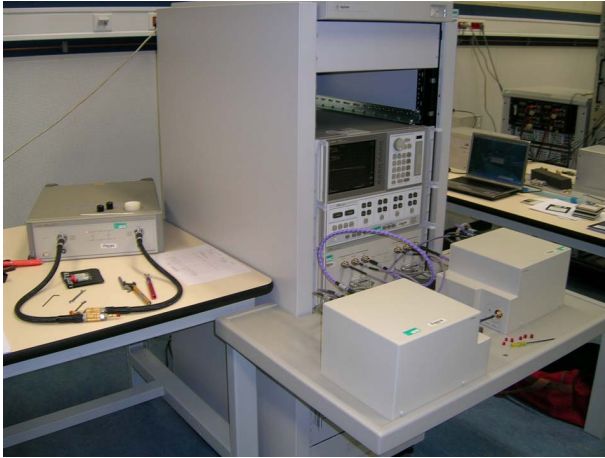
Figure 9. The MVNA of LNE used for the characterization of the satellite simulator's linear components
