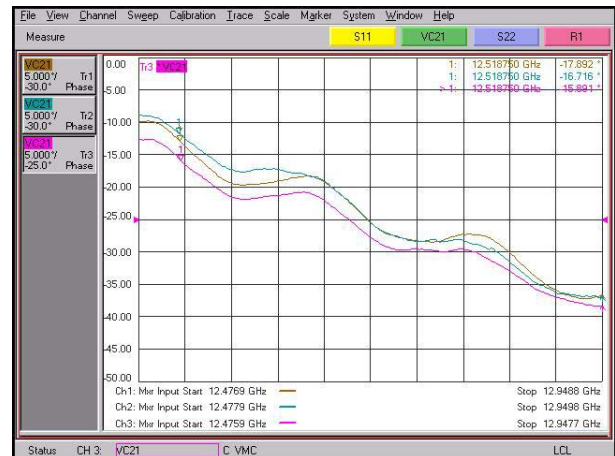
Figure 11. Delay measurement of mixer when the signal is down-converted: a value of 1,2 ns is found
