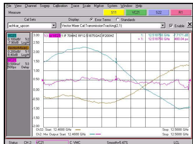
Figure 12. Delay measurement of mixer when the signal is up-converted: a value of 0,5 ns is found
